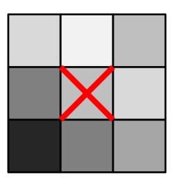
Center pixel has maximum response inside window Center pixel not maximum, suppress
