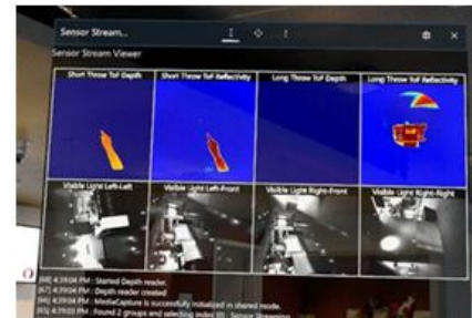
Figure 3: various sensor streams available in Research Mode that could be used to track objects (image Microsoft)
